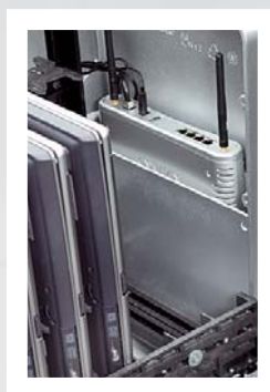
Integrated wireless access point.
